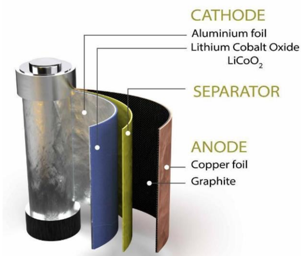
Figure 7. The internal structure of a lithium-ion battery cell. Source: Adapted from Koech et al. [3].
