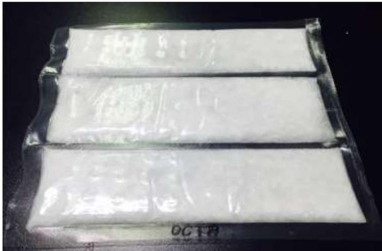
**Fig. 2.** Macro-packed PCM containing n-octadecane.
