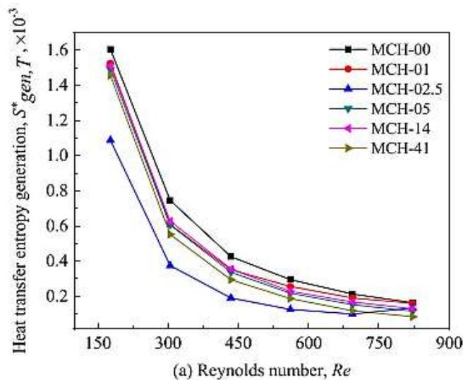
**Fig. 11.** Non-dimensional entropy generation analysis of microchannels with different types as a function of Reynolds number. (a) heat transfer entropy generation  $S^*_{gen, T}$
