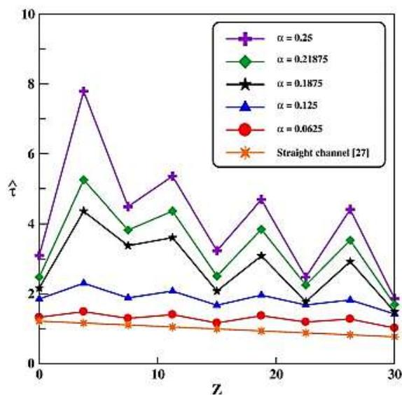
**Fig. 3.** Dimensionless wall shear stress variation along the length of flow direction for both wavy and straight micro-channels.
