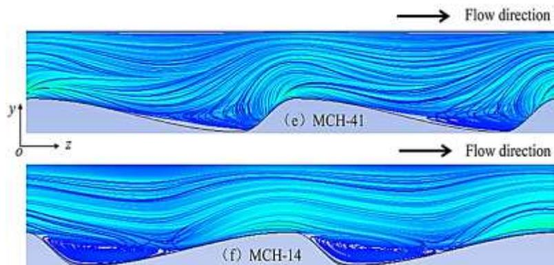
**Fig. 8.** Streamlines of microchannels with different types at  $Re=693$  by numerical simulation. Magnified images of wavy units of MCH-41 and MCH-14.
