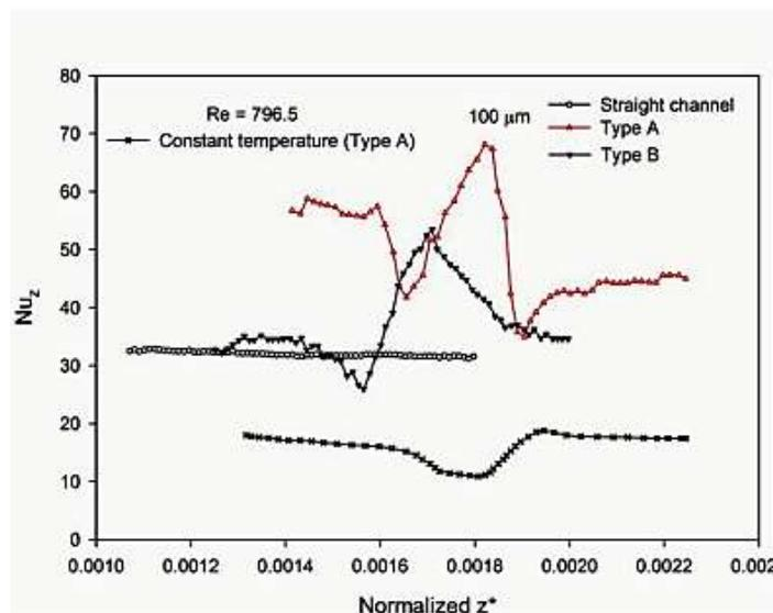
**Fig. 6.** Local Nusselt number along the flow direction in the one of the converging–diverging cross-section.
