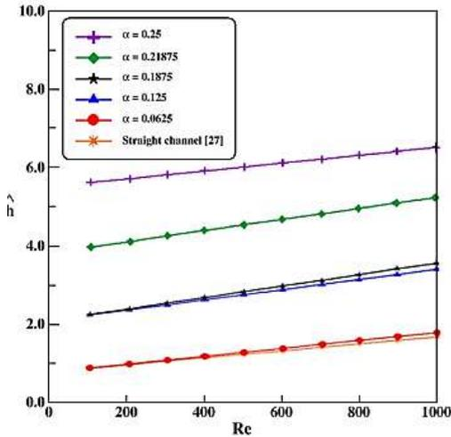
**Fig. 1.** Pressure drop variation versus Reynolds number for both wavy and straight micro-channels.
