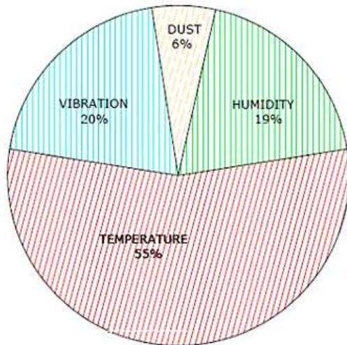
**Fig. 16.** Major causes of electronics failure
