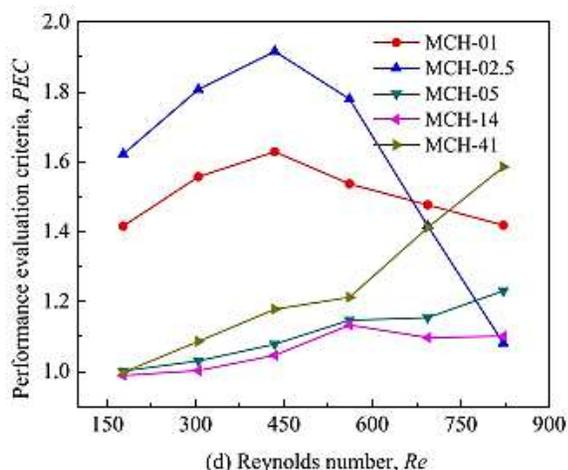
**Fig. 7.** Heat transfer performance of microchannels with different types performance evaluation criteria, PEC, as a function of  $Re$ .
