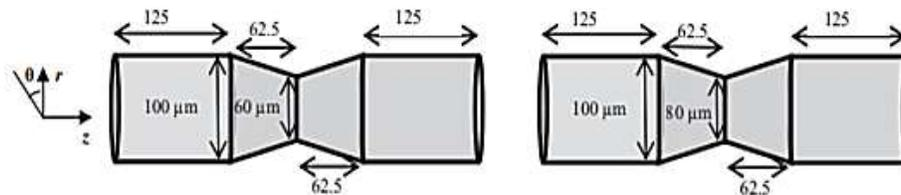
**Fig. 5.** Computational amplitude of one module of converging-diverging cross-section of type A and B channel.
