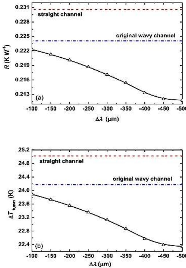
**Fig. 14.** (a) Thermal resistance  $R$  and (b) temperature difference on the bottom wall  $\Delta T_{b,max}$  as a function of  $\Delta\lambda$ .
