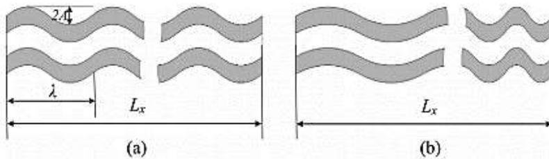
**Fig. 13.** The top view of the wavy channel: (a) original design and (b) new design.
