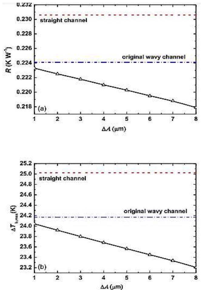
**Fig. 15.** (a) Thermal resistance  $R$  and (b) temperature difference on the bottom wall  $\Delta T_{b,max}$  as a function of  $\Delta A$ .
