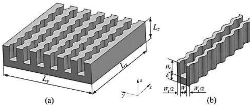
**Fig. 12.** The schematics of (a) wavy microchannel heat sink and (b) its periodic unit.
