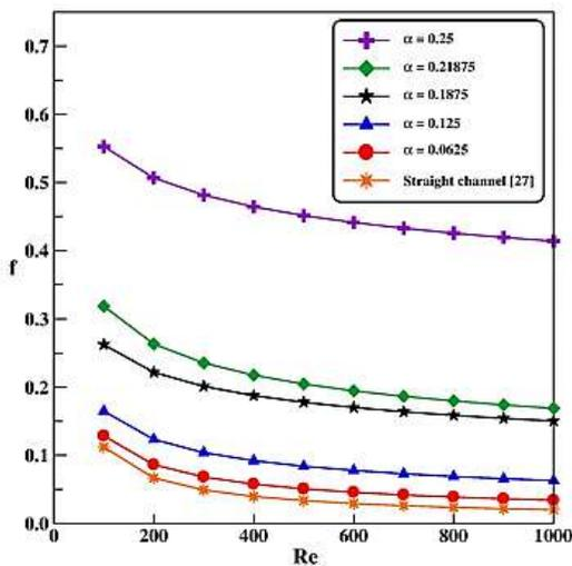
**Fig. 2.** Friction factor variation versus Reynolds number for both wavy and straight micro-channels.
