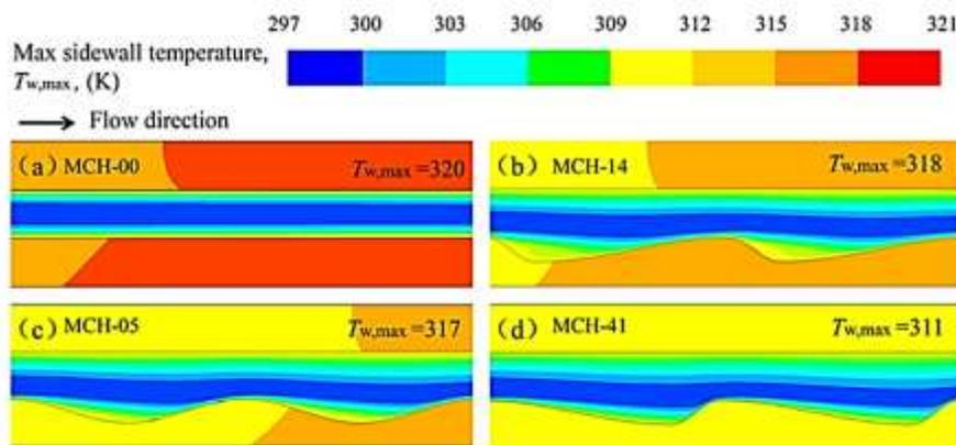
**Fig.9.** Temperature profiles of the sixth and seventh wavy units of the smooth and wavy microchannels at  $Re=434$ .
