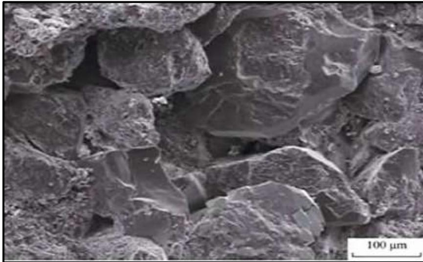
**Fig 9.** SEM images of the core samples before mud circulation [13].
