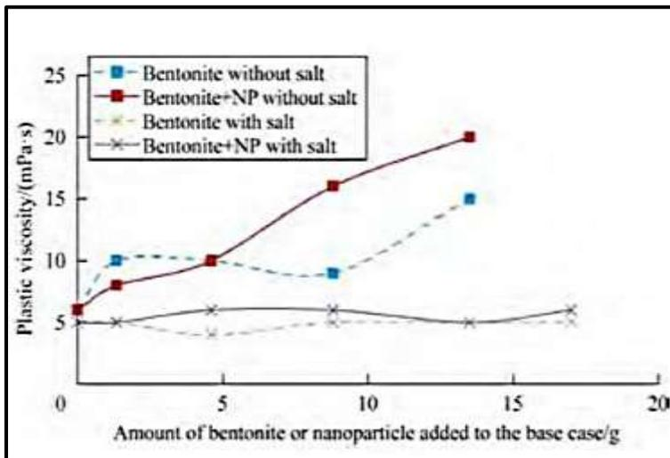
Fig 2. The effect of sepiolite nanoparticles on viscous stains of plastic viscosity [13].
