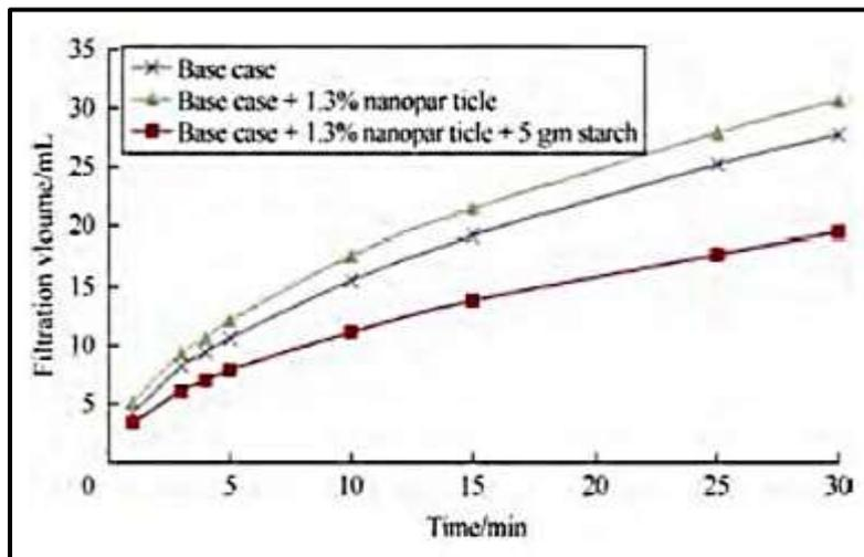
**Fig 5.** Effect of filtration control additive on fluid loss of drilling mud with sepiolite nanoparticles [13].
