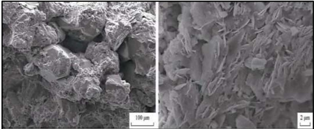
**Fig 12.** SEM images of the core after the circulation of bentonite-based mud without sepiolite nanoparticles (formation side) [13].
