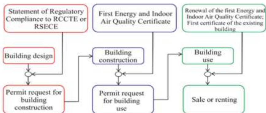
Fig.6. Process to obtain the energy efficiency building label in Portugal, for design, construction and use
