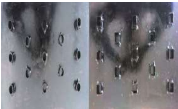
Fig. 8. Pictorial representation of circular (left) and square (right) fins [25].
