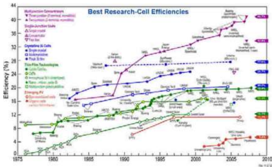
Fig. 4. Trends for efficiency of photovoltaic cells(Rizzo.G,2010).
