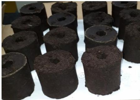
Figure 4. Batch of briquettes made to be tested
