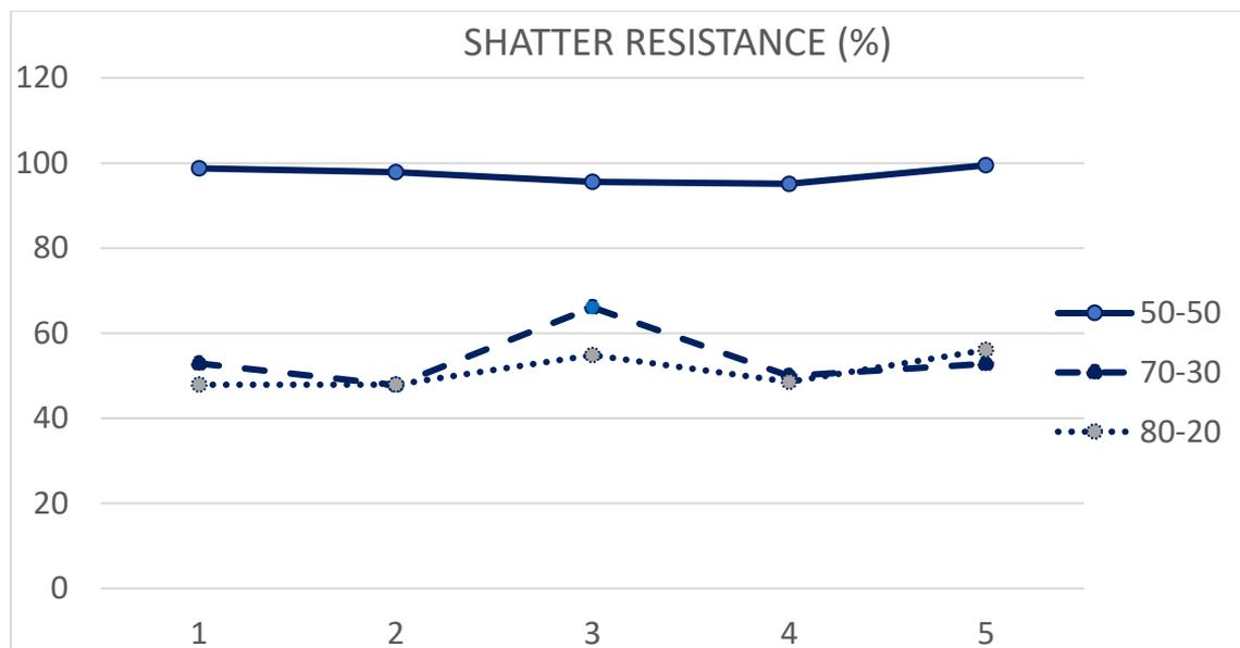
Figure 10. Graphic behaviour of shatter resistance of briquettes SCG-RNP
