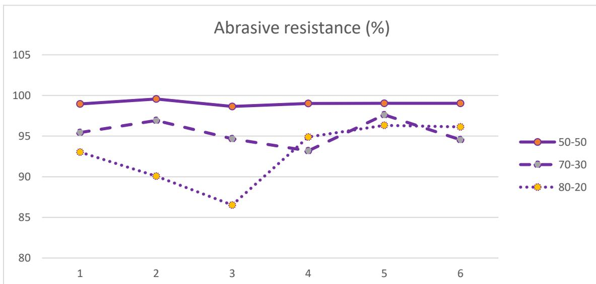
Figure 11. Graphic behaviour of abrasive resistance of briquettes SCG-RNP
