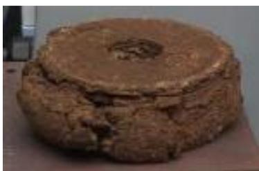
Figure 8. Final appearance of briquette after compression test
