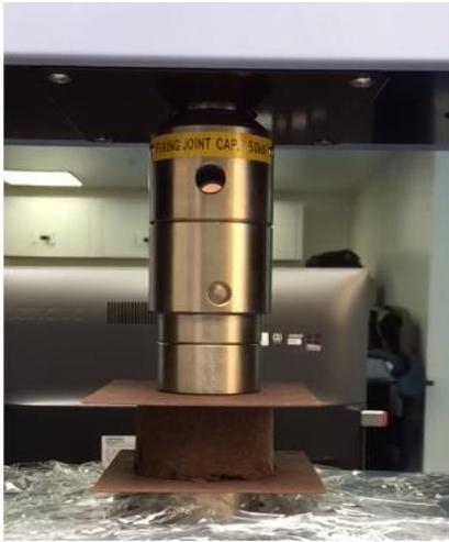
Figure 5. Compression strength test in universal testing machine
