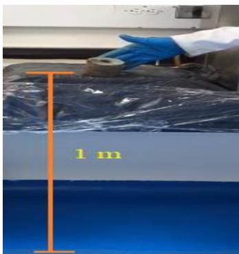
Figure 6. Shatter resistance test
