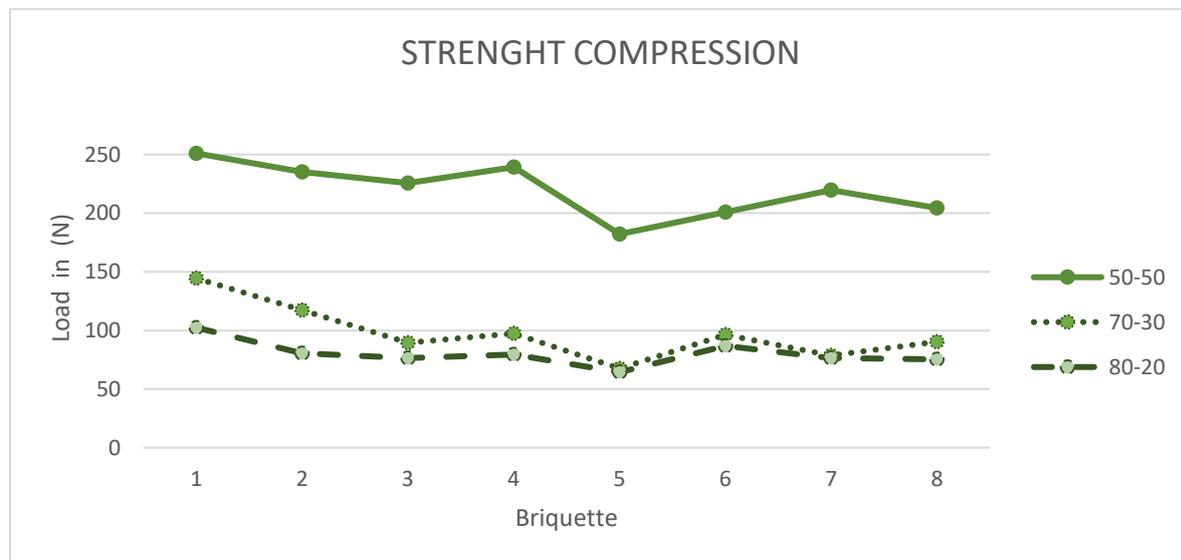
Figure 9. Graphic behaviour of compression strength of briquettes SCH-RNP
