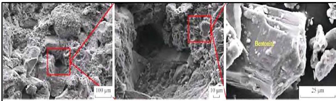
Fig 10. SEM images of the cores after the circulation of bentonite-based mud without sepiolite nanoparticles (wellbore side) [13].
